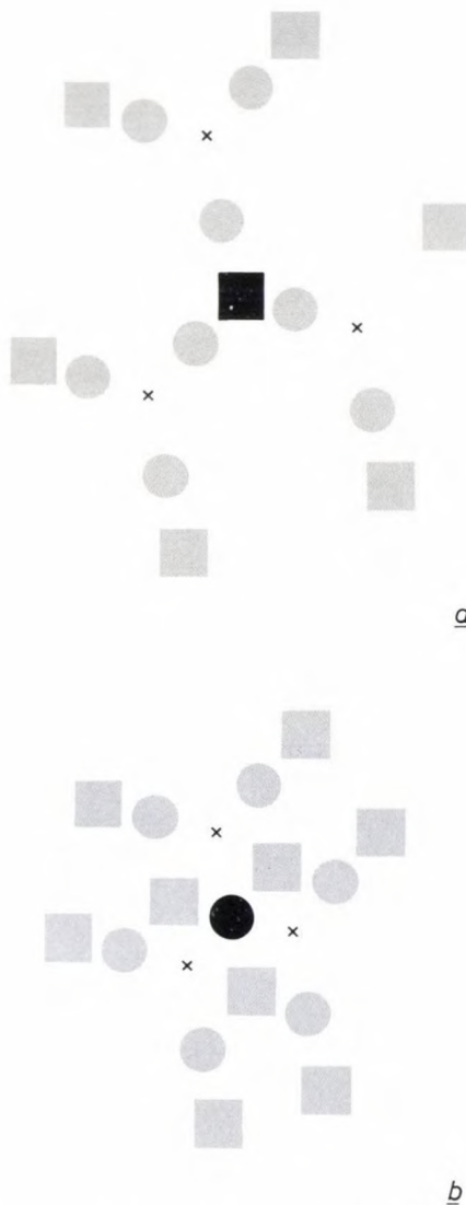
Fig. 3. The decoding. Three projections of the coded image O' of fig. 2 are superimposed after being displaced in such a way that either three squares coincide (a) or three circles (b). The crosses indicate the centres of the three projections. The non-coinciding picture components form a 'noise' background.
