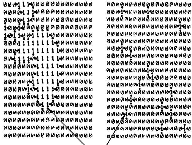
Fig. 11. Principle for calculating the measure of compactness C = T/N for a compact (left) and a diffuse (right) object. T number of transitions (see the arrows) from '1' to '0'. N number of elements of value '1' (object). The regions inside the window have been converted into a binary code by establishing a threshold at a grey level midway between the average at the centre of the window and the average of the boundary points.
