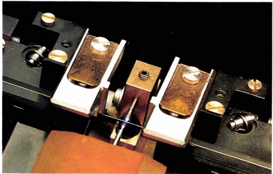
Fig. 2. A closer view of the machine. The arc can be seen at the centre, with glass fibres on either side of it. The fibres are held fast in a V-shaped groove by a spring-loaded clamp (next to the arc). The electrode at the front can be moved towards the one at the back for ignition. There are three height settings for the pair of electrodes. The lowest is the starting position; in the middle position the arc removes the plastic coating, and the actual splice is made in the top position.
