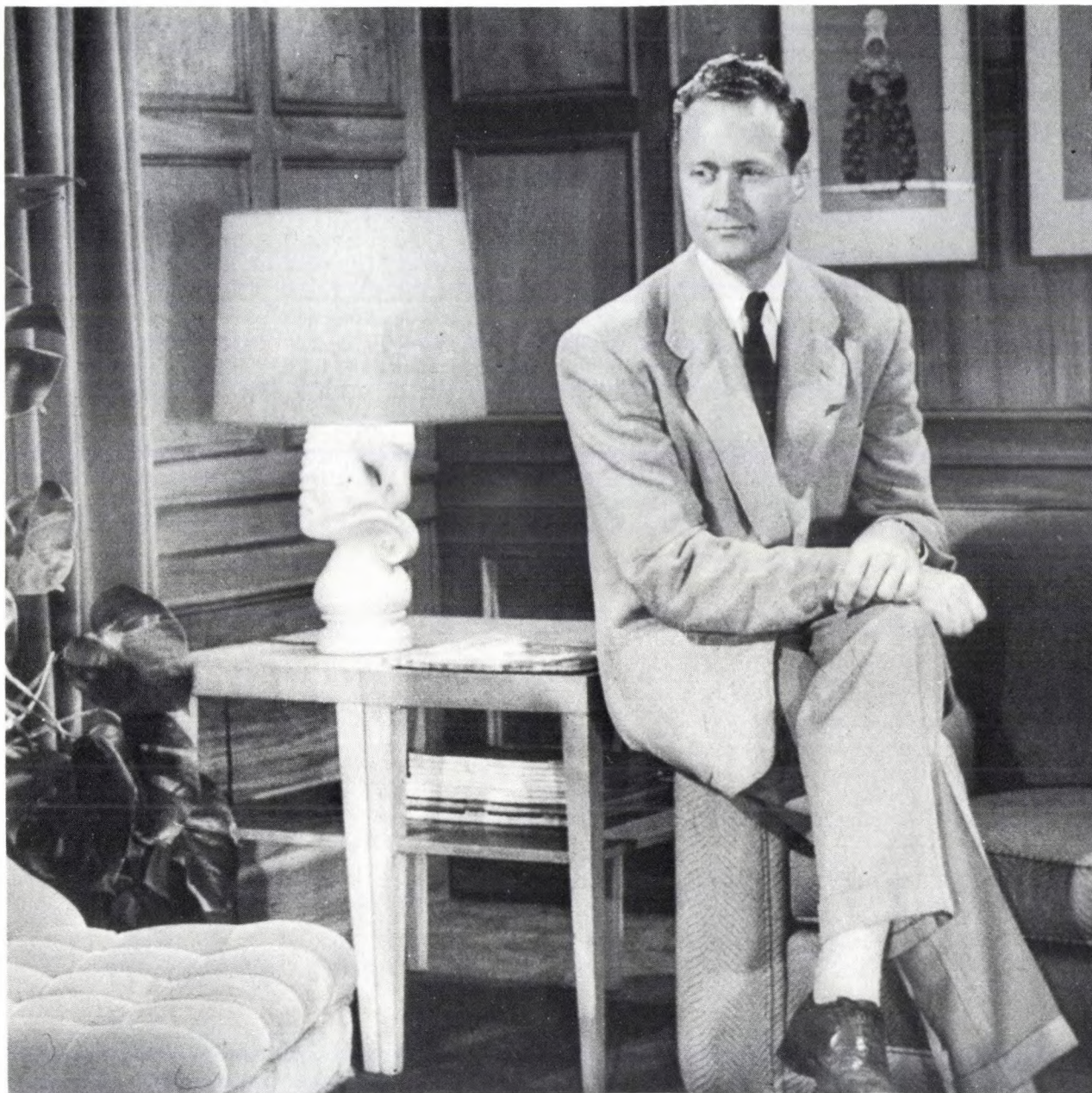
Fig. 4. Illustrating the small effect on picture quality that can be achieved in spite of a considerable reduction in the bit rate, when appropriate coding is used.
